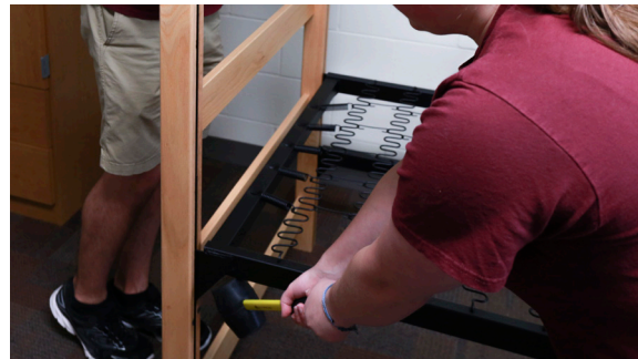
STEP 2 Using the rubber mallet, detach bed spring hooks and stabilizer bar on one side.
